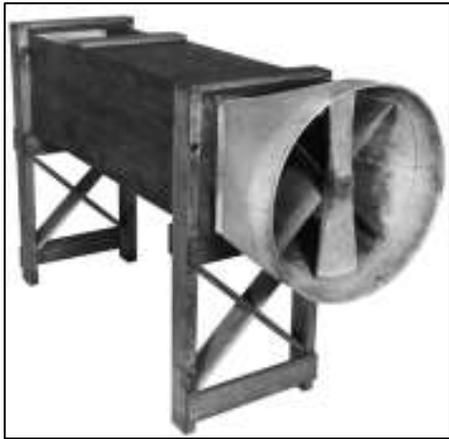
Figura 1. Wright Wind Tunnel [3]
